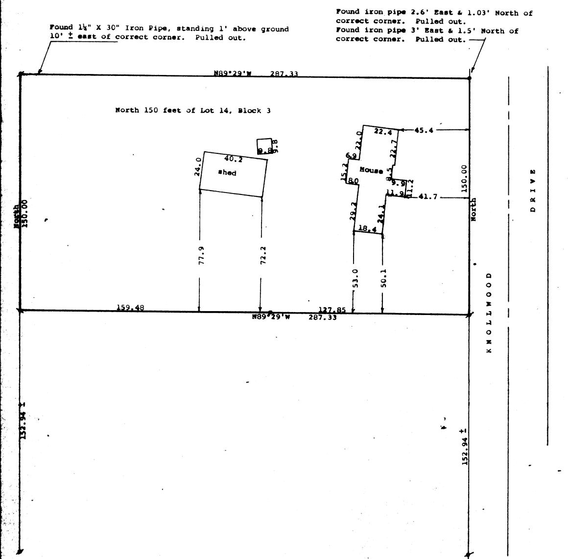
Scale - 1" = 30#= 3/4" Iron Pipe Found " = 1%" Iron Pipe Found up 10" and over a 3/4" Iron Pipe. Reset flush with ground
